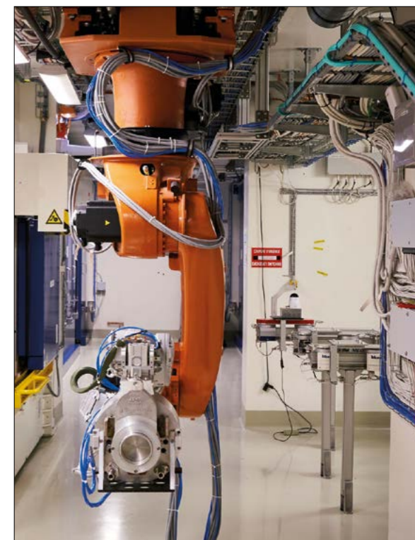
The robot sample handler at MEDICIS, a unique facility for the production of unconventional isotopes.
