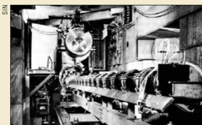
The long superconducting solenoid at the SIN cyclotron has yielded the world's highest fluxes of muons.
