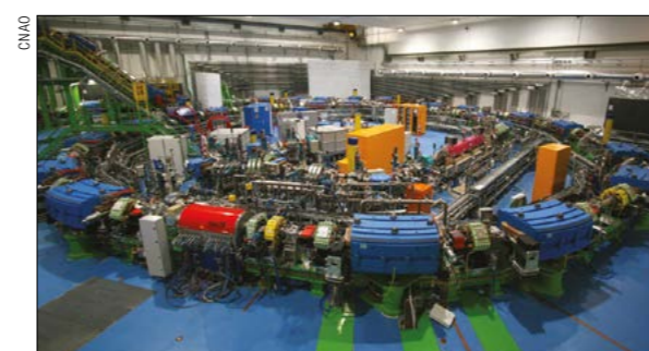
The 25-m-diameter synchrotron of CNAO in Italy.
